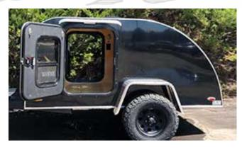
This rugged off-road trailer will get you off the beaten path in comfort. Based on our Queen size platform, same strong aluminum welded frame but with a full skid plate, heavy duty torsion axle to support off-road BF Goodrich All-Terrain T/A KO2 15" tires..
